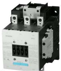
CONTACTOR, 75KW/400V/AC-3, AC(40...60HZ)/DC OPERATION UC 200...277V AUXIL. CONTACTS 2NO+2NC 3-POLE, SIZE S6 BAR CONNECTIONS ELECTRONIC OPERATING MECHANISM WITH PLC INTERFACE 24V DC SCREW TERMINAL
